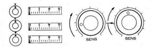
When measuring an unknown inductance, seek the proper range by turning the dials and "LOSS BALL" knob.
