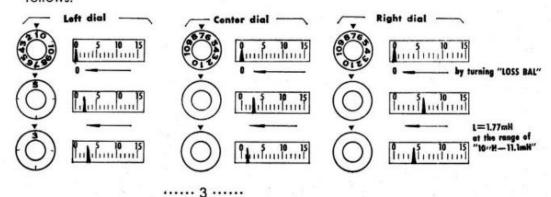
Note: When the meter pointer !ndicates "0" on two or three positions of the dial by turning "LOSS BAL" knob, turn "SENS" knob slightly to the right and continue the measurement.
